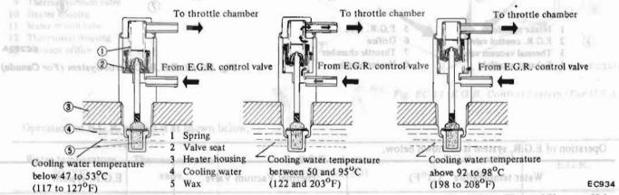
Fig. EC-14 Thermal Vacuum Valve
