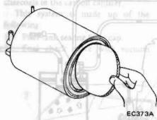
Fig. EC-40 Replacing Carbon Canister Filter
