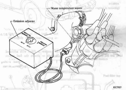
Fig. EC-33 Connecting Emission Adjuster
