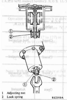
Fig. EC-9 Adjusting B.C.D.D.
