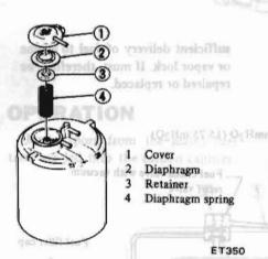
Fig. EC-39 Carbon Canister Purge Control Valve
