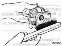
Fig. EC-27 Cleaning E.G.R. Control Valve (23 to 31 ft-lb)
