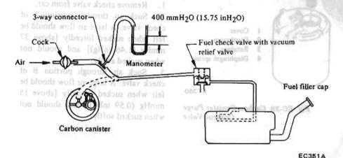
Fig. EC-37 Checking Evaporative Emission Control System
