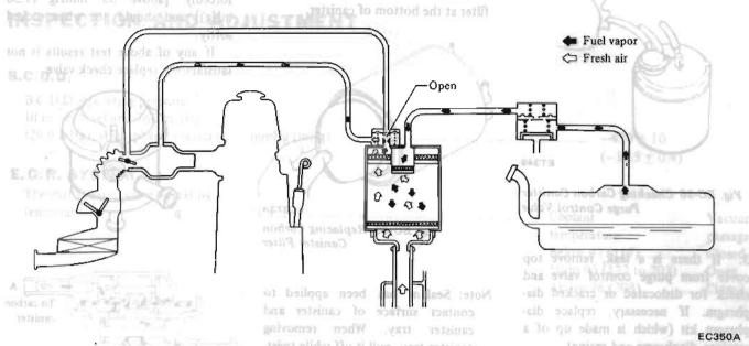
Fig. EC-36 Evaporative Emission Control System (Fuel vapor flow when engine is running)
