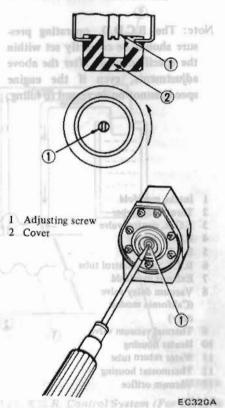
Fig. EC-10 Adjusting B.C.D.D. Operating Pressure (Non-California models)
