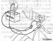
Fig. EC-6 Checking Vacuum Control Solenoid Valve
