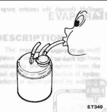
Fig. EC-38 Checking Carbon Canister Purge Control Valve
