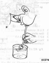
Fig. EC-24 Checking Vacuum Delay Valve
