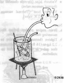
Fig. EC-22 Checking Thermal Vacuum Valve
