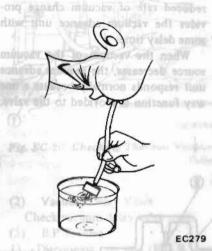
Fig. EC-30 Checking Vacuum Delay Valve
