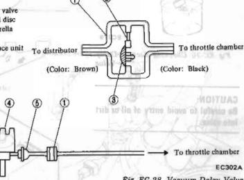
Fig. EC-28 Vacuum Delay Valve
